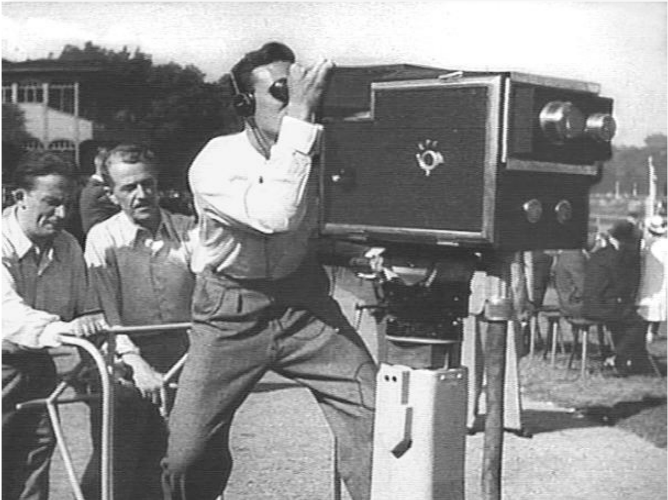
A German twin lens Fernseh Iconoscope television camera.
